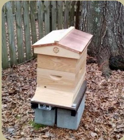
The primary element of the **B-ware™ Beehive Monitoring System** is the **B-ware™ Smart Hive Monitor**. The Smart Hive Monitor measures and stores weight and temperature readings every 15 minutes. These readings are very precise and can measure even very slight changes in beehive weight. Hive monitors can be read either with a handheld device such as a smartphone or remotely and automatically using a B-ware™ Data Collector.
